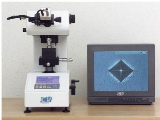
Figure 1. Micro-Vickers Hardness Tester, 400-DM, CV Instruments
