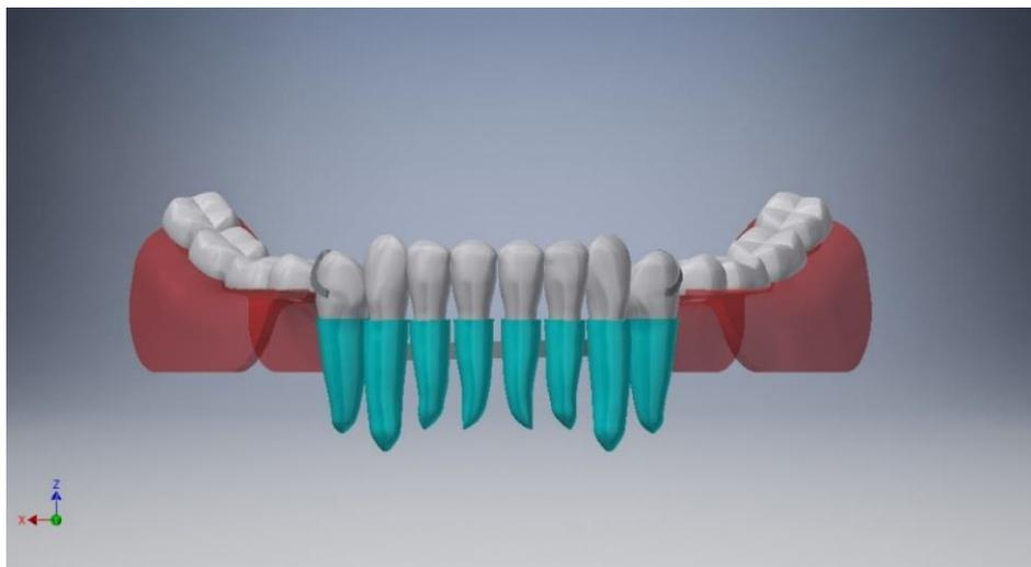
**Figura 1.c.** Metallic removable denture with « Ackers » clasps
